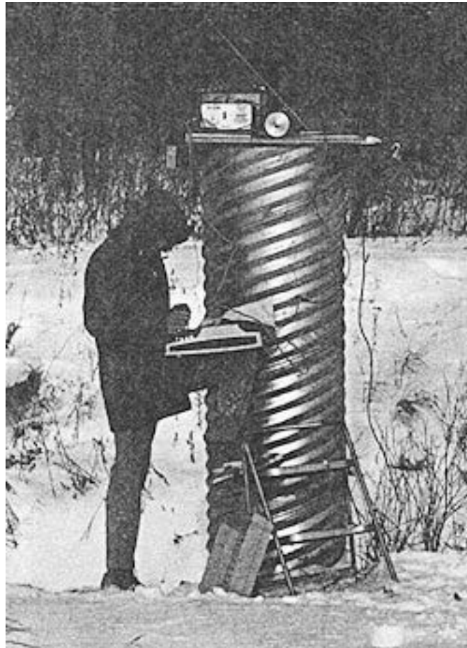
Staff regularly monitor the Kintore Creek watershed to estimate the amount of eroded soil reaching the stream.
