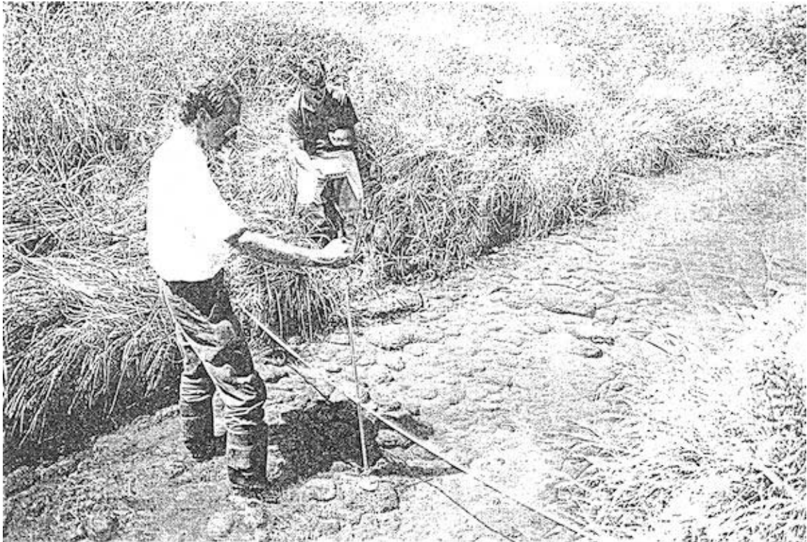
Fig 7: A current meter is used to calculate stream velocity in low flow conditions.
