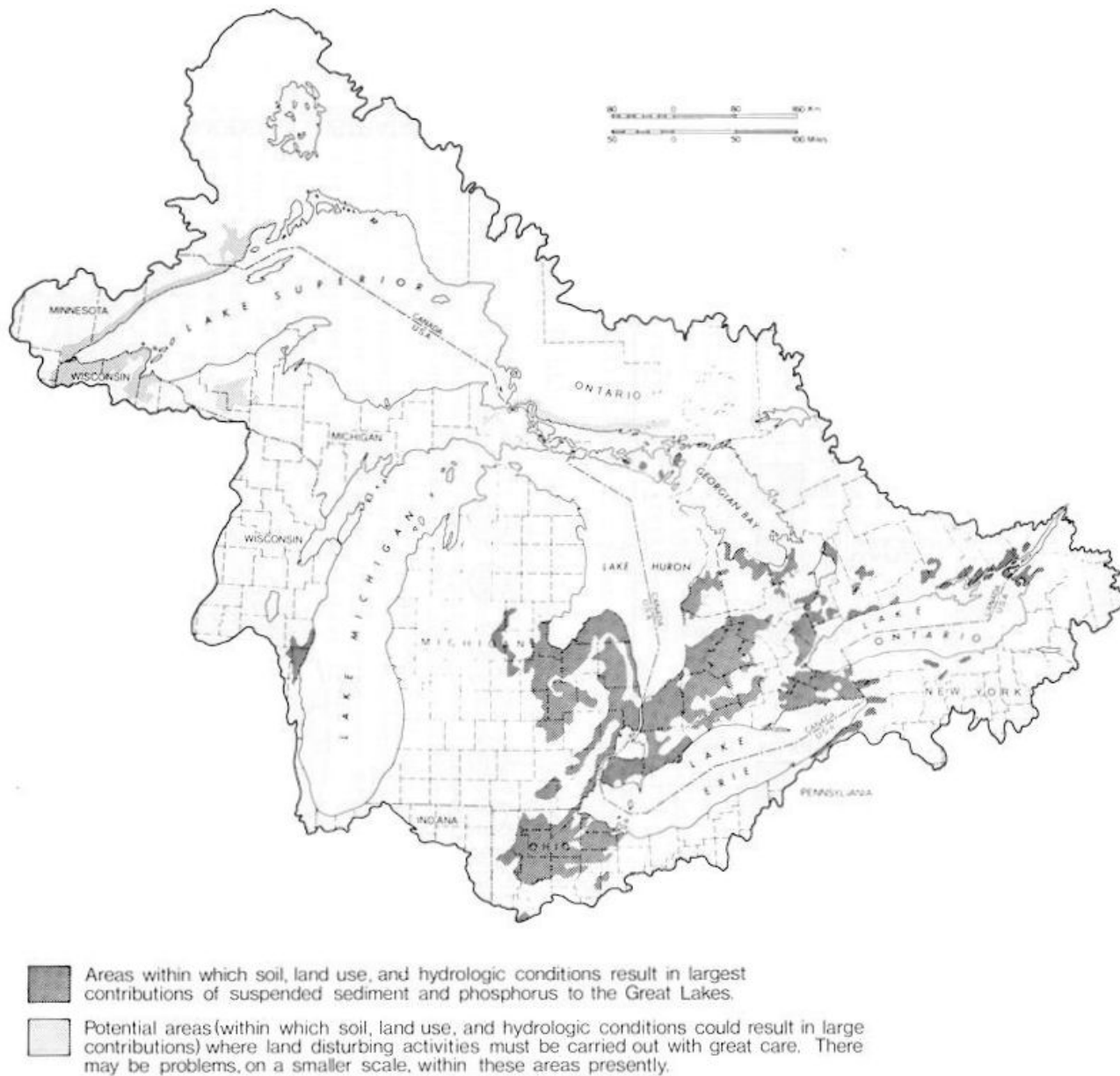
FIGURE 1: Regions Of Fine Textured Soils Requiring, Or Potentially Requiring Treatment For Erosion Control
