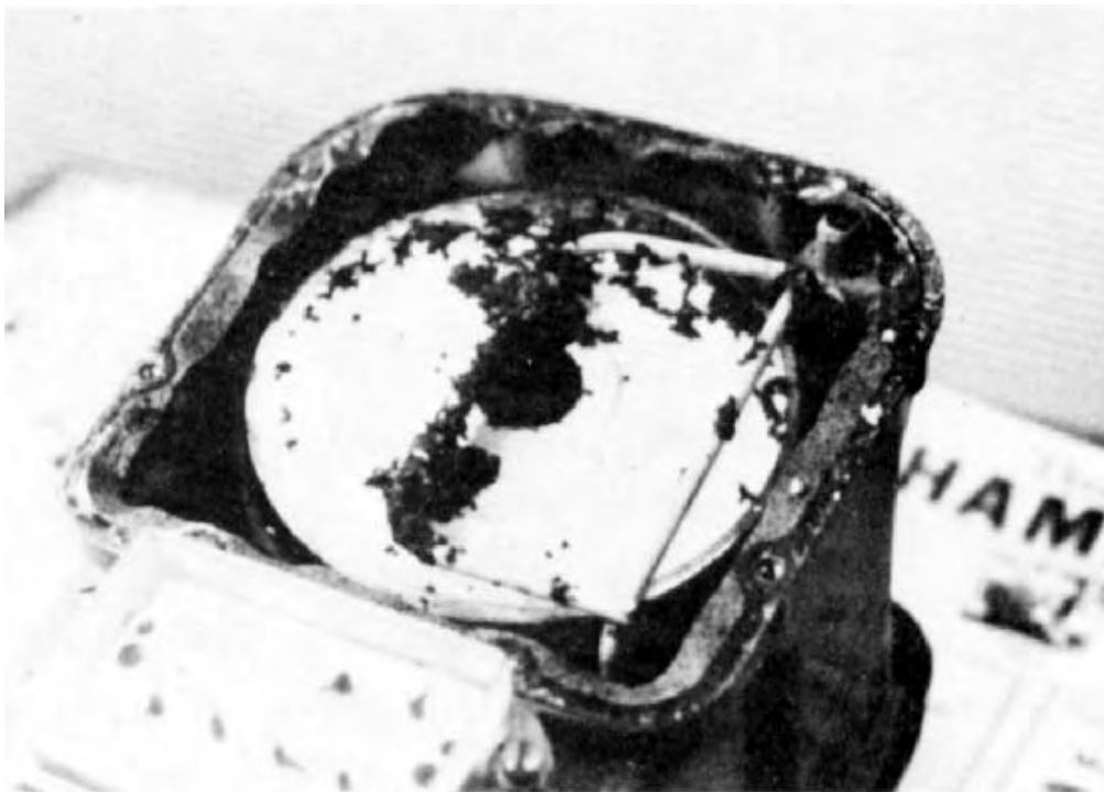
Figure 3. Corrosion of a gas meter after one year of operation
