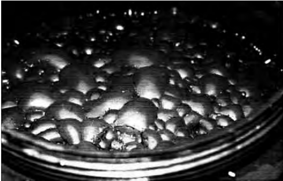
Plate 6. Slurry surface inside the barrel after filling; a nine-inch free space was left above the slurry.
