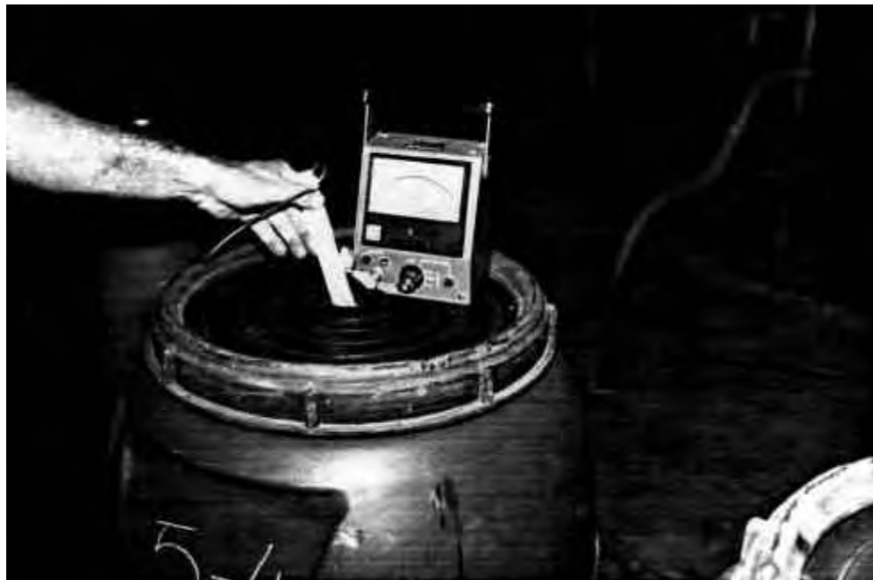
Plate 11. Determining slurry temperature.
