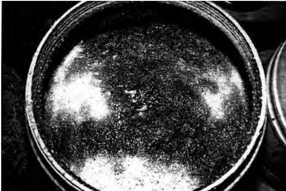
Plate 15. Typical surface appearance of unmixed slurry at the end of 10 week storage period in all treatments, including control, except peat and hydrogen cyanamide.
