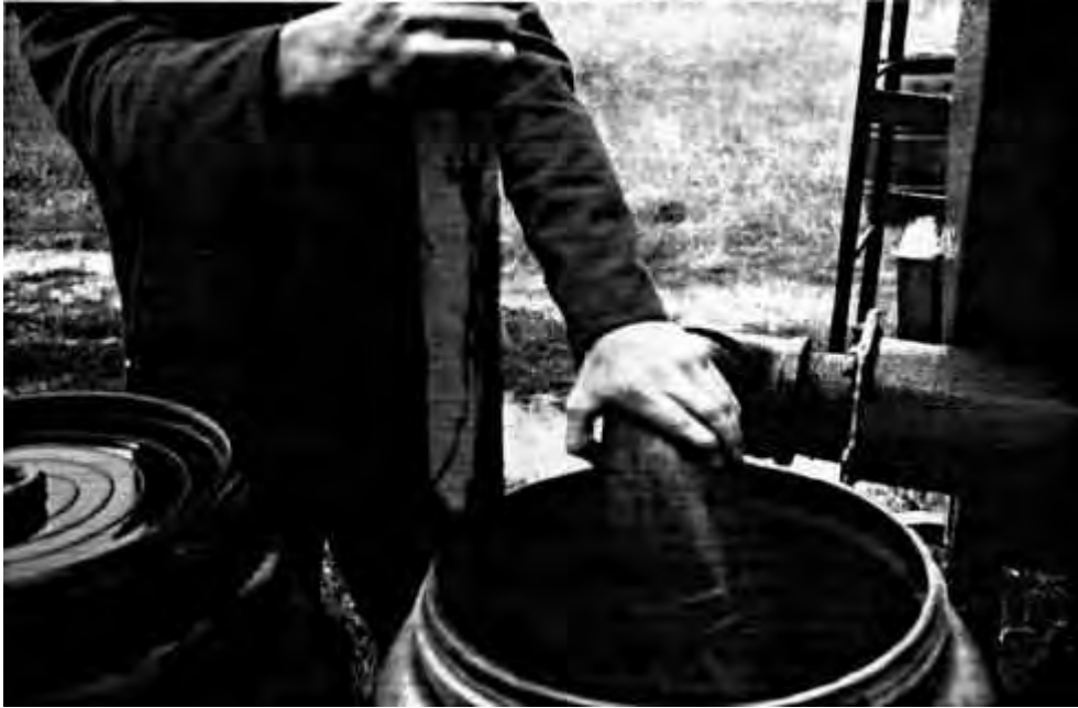
Plate 5. Filling test barrel with a fixed volume of slurry.
