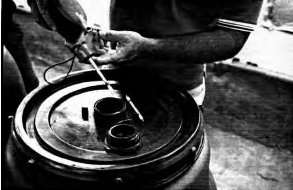
Plate 10. Testing for gas concentration in the free space inside the barrel.
