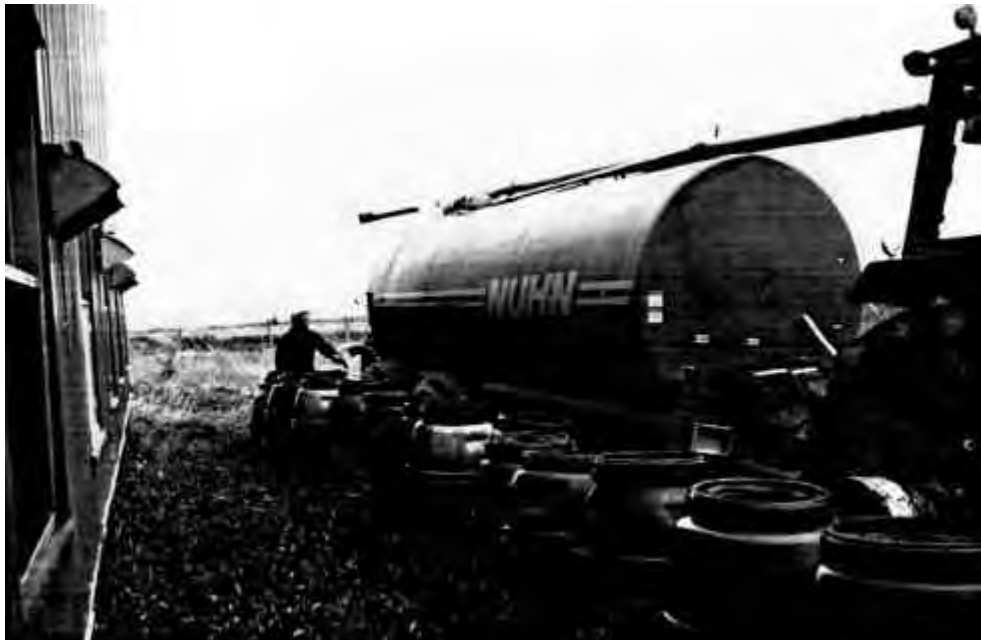
Plate 4. Aligning tanker discharge pipe to barrel opening.
