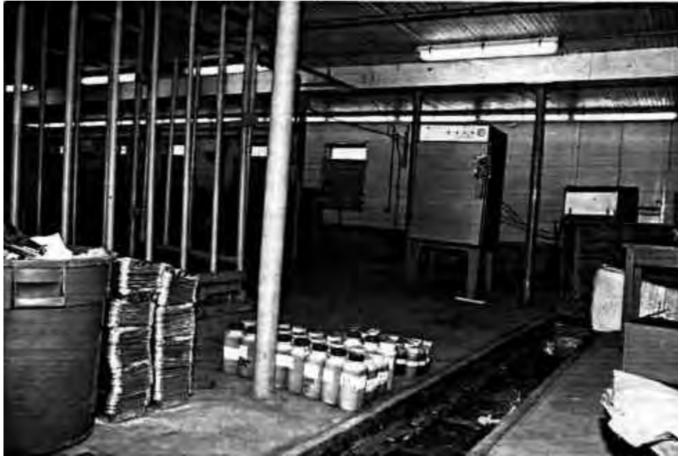
Plate 12. Drying oven used in the barn for slurry dry-matter determination.
