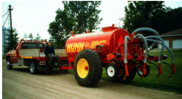
Figure 8. A "Manure Research Unit" built by Nuhn Industries to test direct injection techniques for swine manure.
