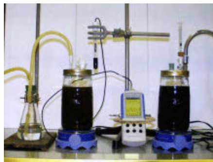
Fig. 6 - Manure is being incubated with (left) and without (right) aeration.
