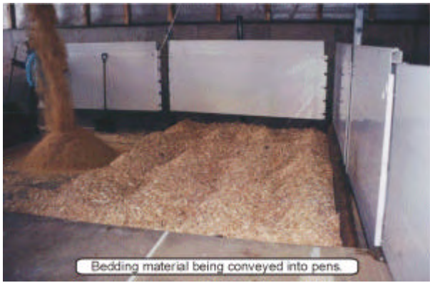
Mixer wagon with load cells weighing and mixing bedding components. Conveyor for moving bedding into pens.
