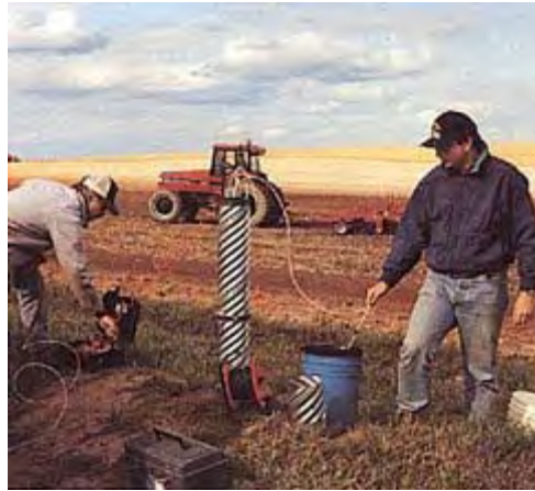
Monitoring a well for groundwater quality in land under potato production in Atlantic Canada.
